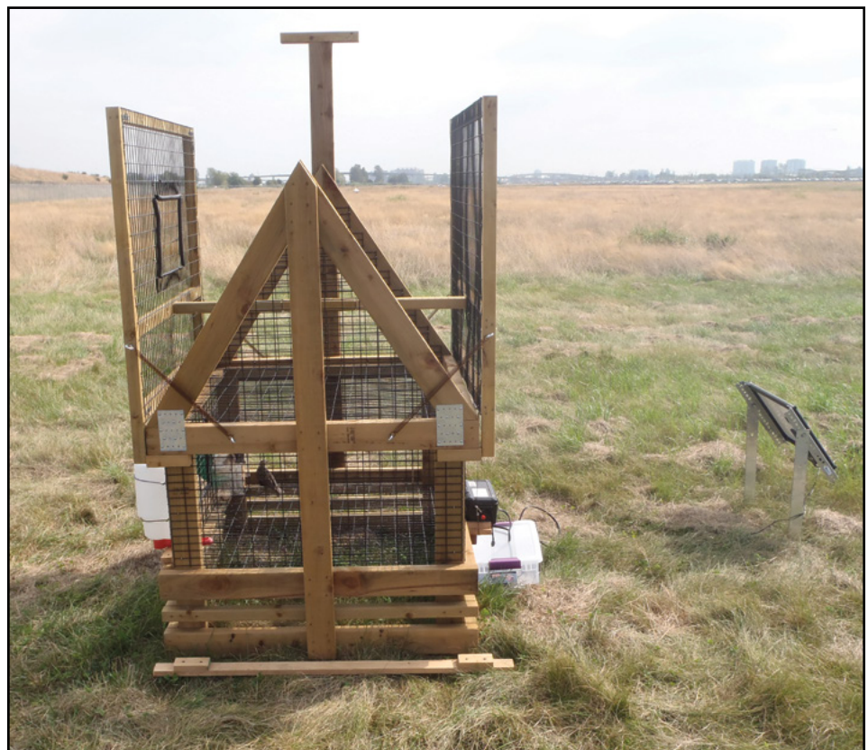
Swedish Goshawk Trap equipped with TrapSmart system and solar charger.
