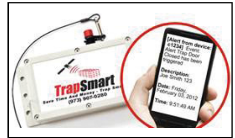
Figure 1: TrapSmart sends a text alert to your mobile when the trap fires.
